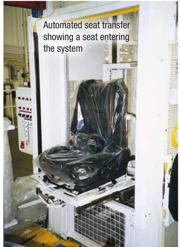
Automated seat transfer showing a seat entering the system
