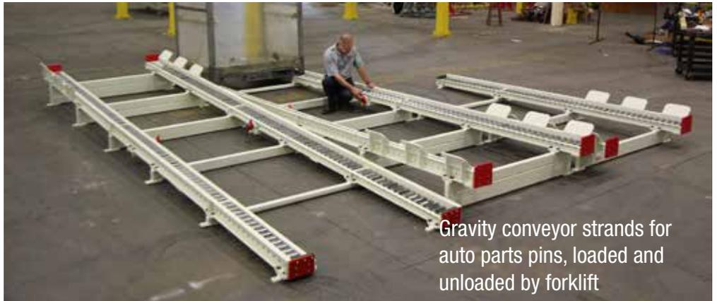
Gravity conveyor strands for auto parts pins, loaded and unloaded by forklift
