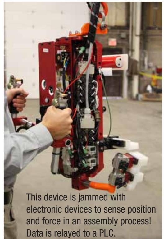
This device is jammed with electronic devices to sense position and force in an assembly process! Data is relayed to a PLC.
