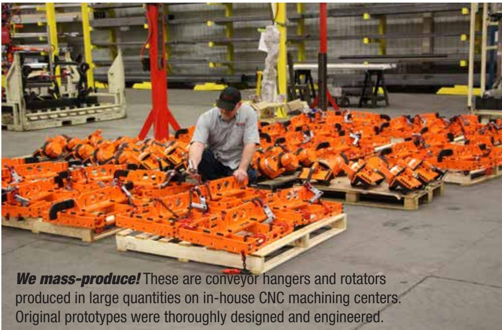
**We mass-produce!** These are conveyor hangers and rotators produced in large quantities on in-house CNC machining centers. Original prototypes were thoroughly designed and engineered.
