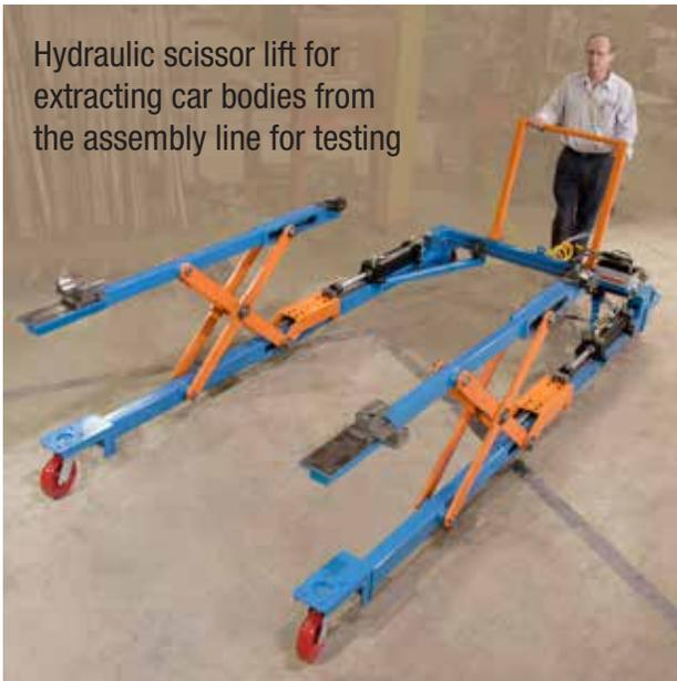
Hydraulic tandem lift platforms for auto assembly line workers
