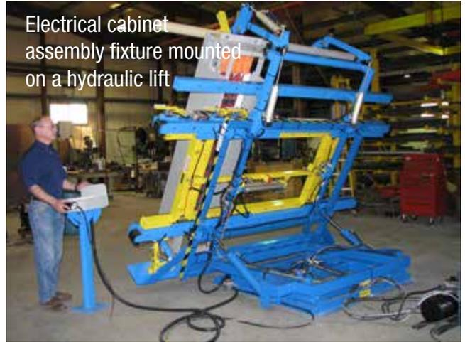
Electrical cabinet assembly fixture mounted on a hydraulic lift
