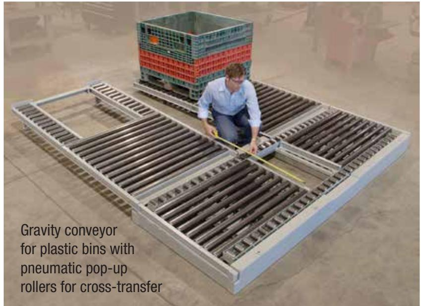
Gravity conveyor for plastic bins with pneumatic pop-up rollers for cross-transfer
