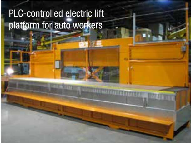
High-speed electric lift platform: extremely rigid upper deck with no flex and no sway (plywood deck removed for clarity)
