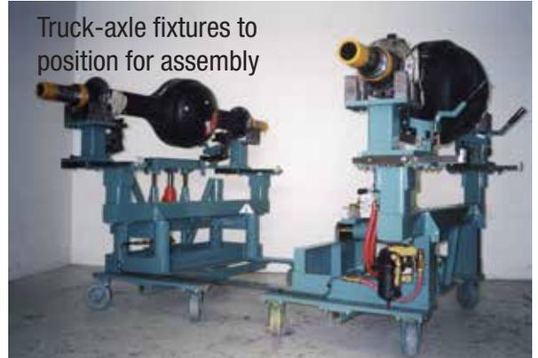
Truck-axle fixtures to position for assembly
