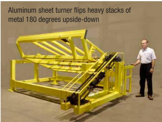
Aluminum sheet turner flips heavy stacks of metal 180 degrees upside-down
