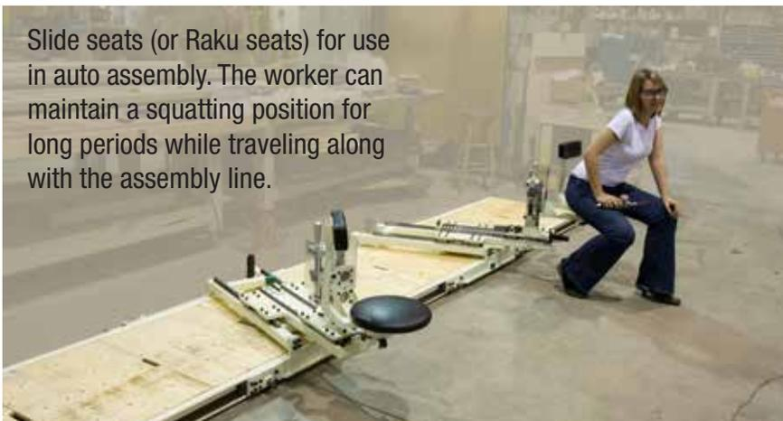
Slide seats (or Raku seats) for use in auto assembly. The worker can maintain a squatting position for long periods while traveling along with the assembly line.
