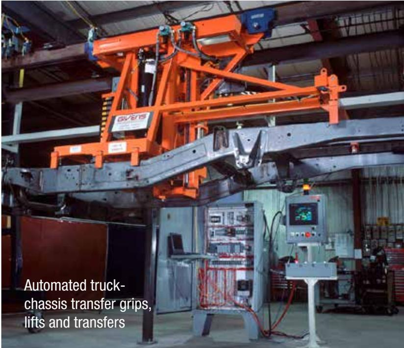
Automated truck-chassis transfer grips, lifts and transfers
