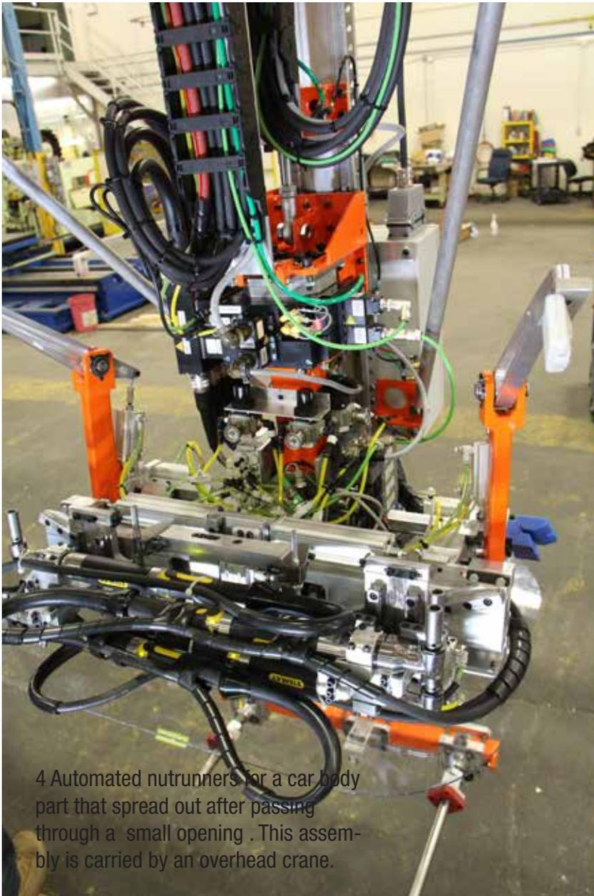
4 Automated nutrunners for a car body part that spread out after passing through a small opening. This assembly is carried by an overhead crane.
