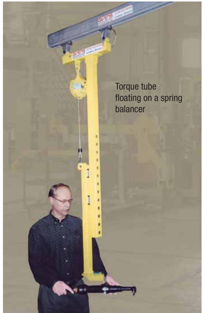
A torque tube supporting 2 nutrunners. Note that the right-angle nutrunner drives against a fork that prevents a nut from turning, at the bottom.
